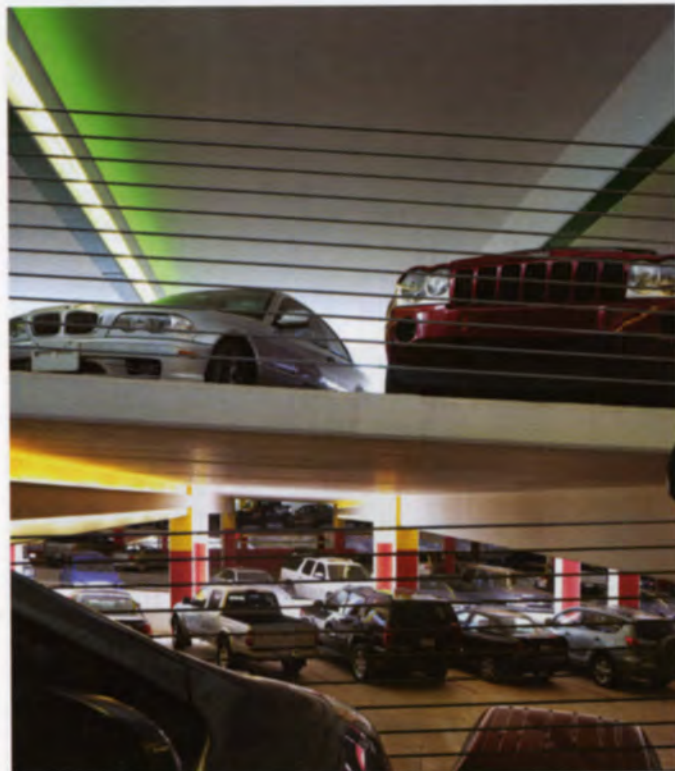
Colored lighting instantly tells drivers the color code of the floor on which they parked.
